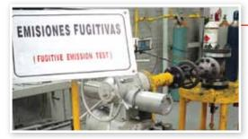
**Low Fugitive Emissions Test**. This test is performed when a Customer requires low fugitive emissions certification. Our Lab has its own LFE test equipment that is capable of measuring less than 20 ppm in both static and mechanical conditions at either ambient temperature or thermal cycle operations.
