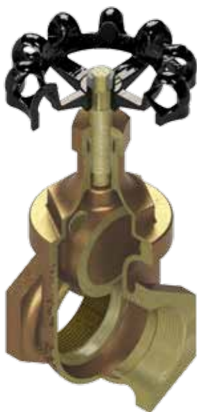
Solid Wedge Bronze as per ASTM B62 C83600 for non-rising stem (only for W4 and W14)
