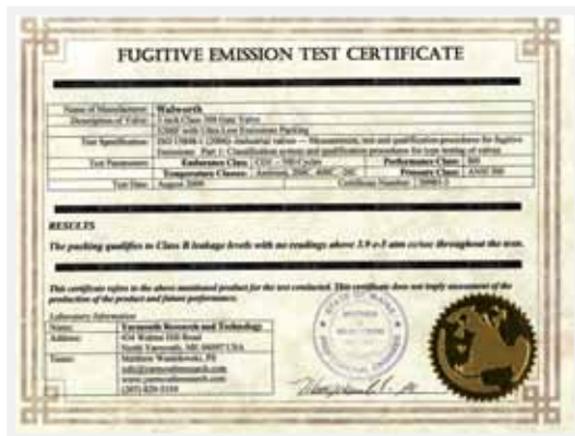
Emissions after 500 cycles at ambient and 350 °F Issued by Yarmouth Research and Technology Lab for 3 inch Class 300 Gate Valve After 500 cycles the measurement result was less than 50 ppm.
