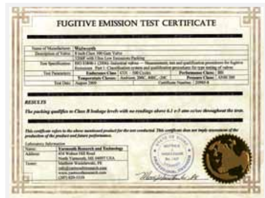
Emissions after 500 cycles at ambient and 350 °F Issued by Yarmouth Research and Technology Lab for 8 inch Class 300 Gate Valve After 500 cycles the measurement result was less than 50 ppm.
